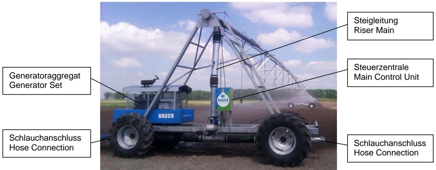
The *main cart (central unit)* consists of the following components:
